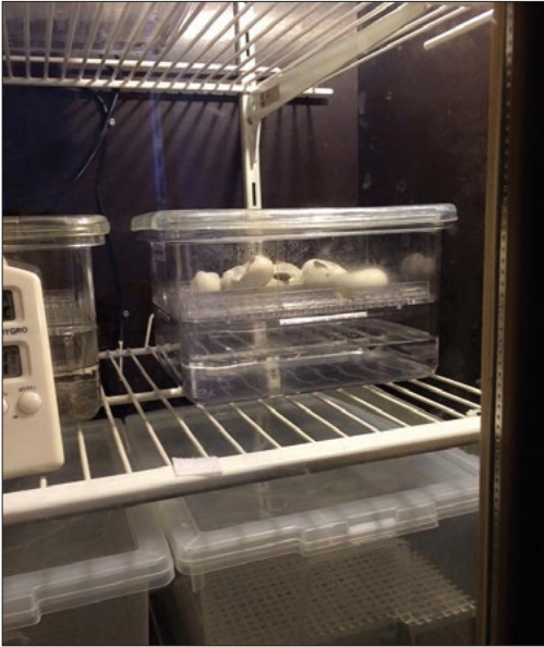
Figuur 10. De broedstuf met daarin de broedbox. Figure 10. The incubator with the incubation box in it.
